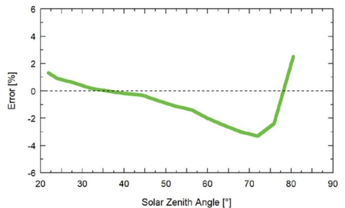
Mean cosine response of four Apogee SE photometric sensors. Cosine response was calculated as the relative difference of SE photometric sensors from the mean of replicate reference photometric sensors deployed outdoors. These data are the average of the AM and PM response.
