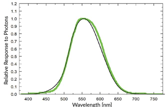
Spectral sensitivity of photometric sensors. Replicate (n=6) sensors indicate a spectral shift to lower wavelengths caused by non-zero incidence angle, resulting in mismatch between CIE 1931 photopic weighting factors and sensor sensitivity. Measurements were made with CR6 datalogger at 10 nm increments in the monochromator.
